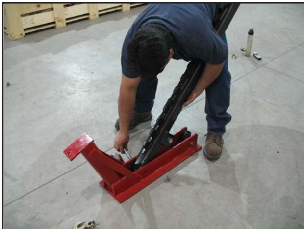
Attach post to base using supplied nut & bolt.
