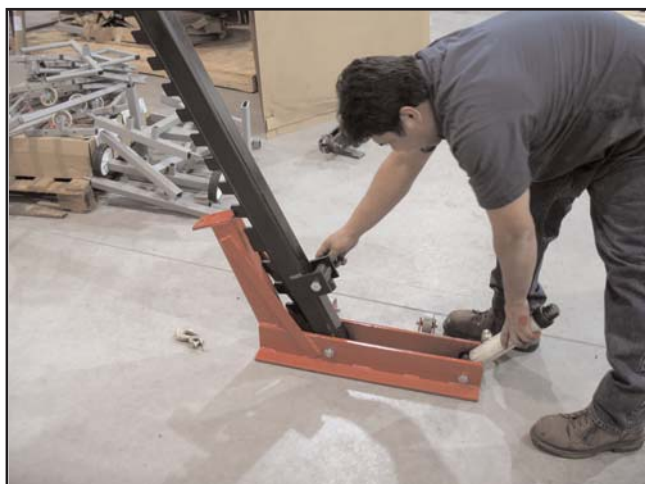
Remove bolt from ram coupler on post.c
