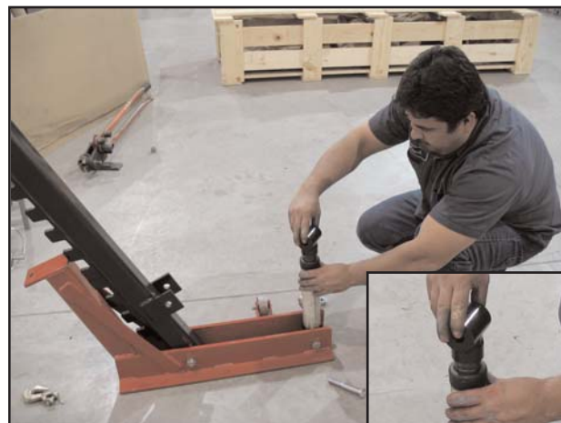
Screw ram coupler onto top of hydraulic ram.
