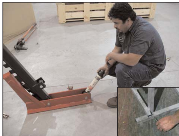
Screw hydraulic ram onto ram coupler at end of base. Hydraulic ram may or may not be included depending on which package you buy.
