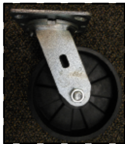
SWIVEL CASTER 6" DIAMETER WHEEL 7 1/2" MOUNT HT. LOAD CAPACITY 1200 LBS PER WHEEL (2) REQ'D
