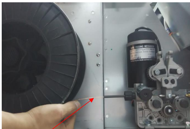
(2) Note the tension spring adjuster and spool locating pin.
