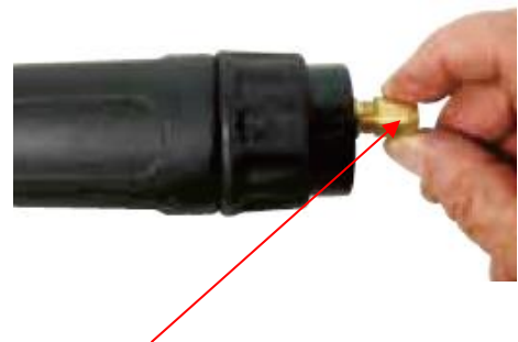
(6) Fit the liner retaining nut and screw only 1/2 way down.
