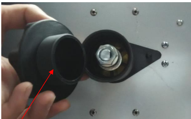
(1) Remove the spool retaining nut.
